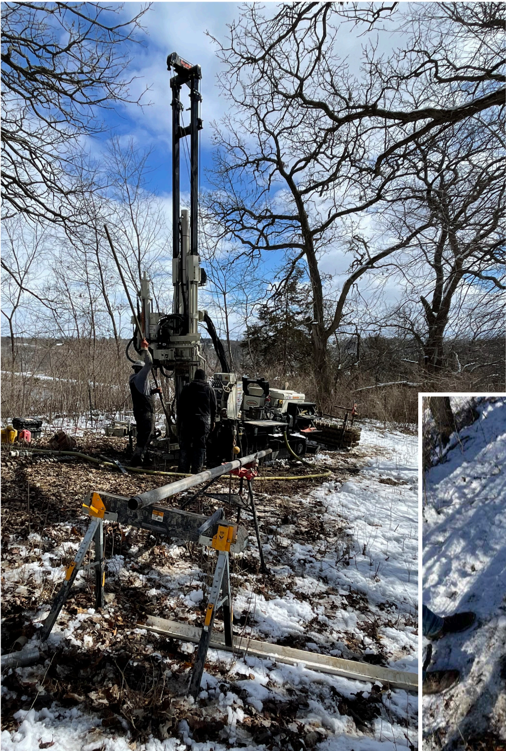
The Rubino engineers used a Geoprobe rock borer to obtain rock core samples so that they could run structural tests on the rock for the spillway project.
