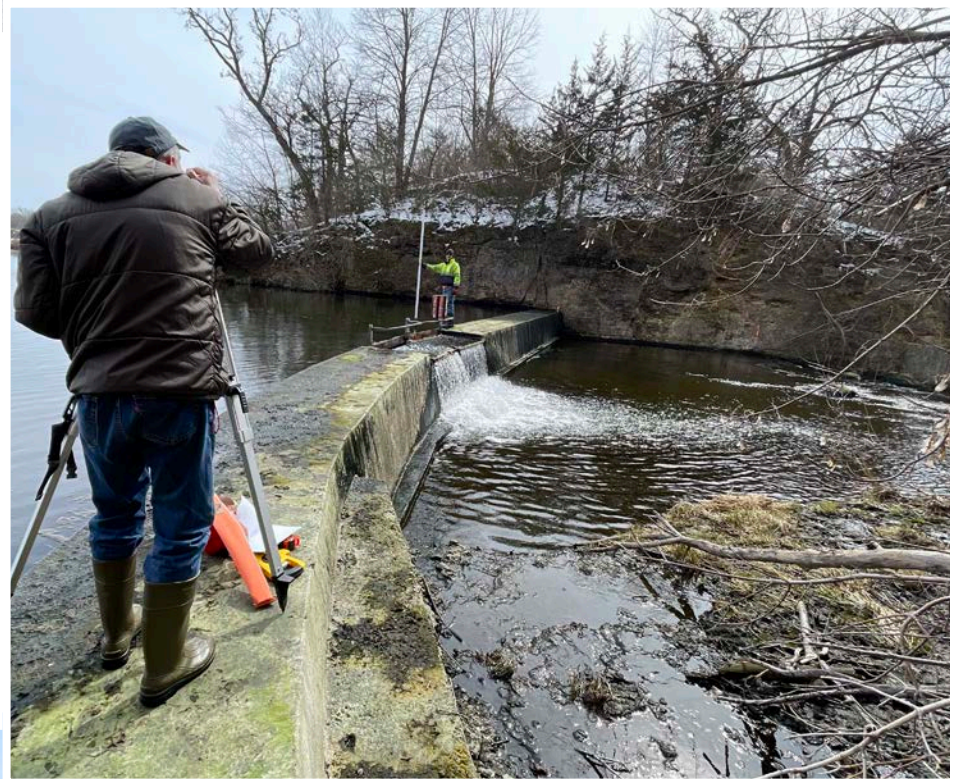
ABOVE: CMT engineer Ted LaBelle and Natural Resource Manager Tyler Hesselbacher take elevation measurements throughout various points on the weir and channel.
