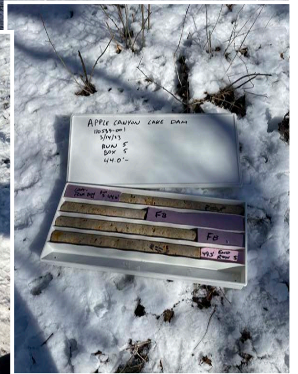
Left and Above: Rock core samples that will be run through various structural analyses.
