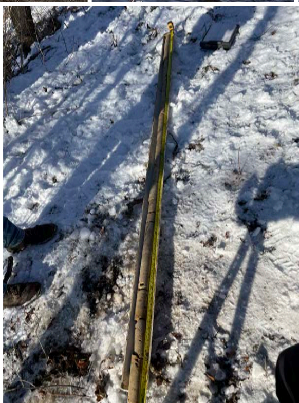
The Rubino engineers used a Geoprobe rock borer to obtain rock core samples so that they could run structural tests on the rock for the spillway project.
