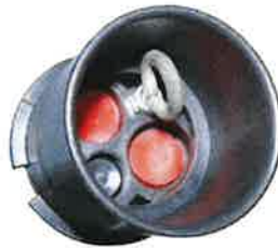
Bottom View shows eyebolt used to secure pumps and Leveloggers
